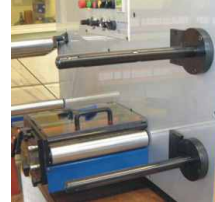
Twin rewinds (air shafts)
